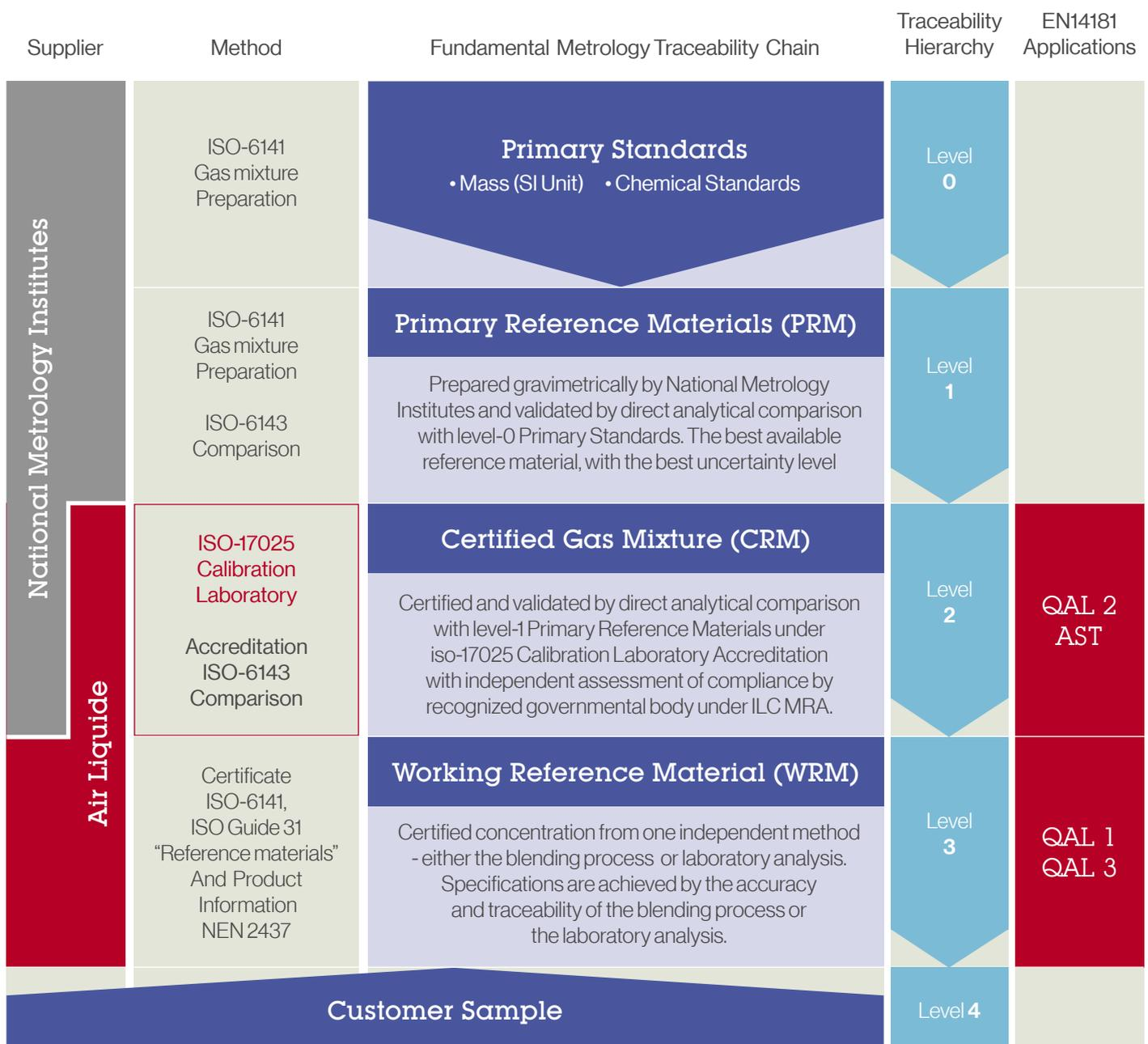
This uncertainty measurement is very important with regards to adhering to the standard reference methods (SRMs) whilst conducting QAL2 and AST procedures.
